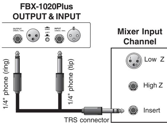
**Note:** If you're using a mixer with unbalanced 1/4" outputs, you must use standard unbalanced cables and connectors when connecting it to the FBX. Similarly, if your mixer is wired for balanced 1/4" (Ring/Tip/Sleeve) outputs, you must use that type of connector. If you don't, you may experience a loss of gain when using the FBX.
